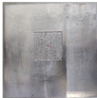
图7 激光喷丸处理后试件 Fig.7 A laser-treated test piece
